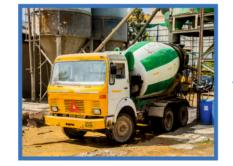
TRANSIT MIXTURE Greaves Cotton - 6m3 drum capacity Schwing Stetter - 6m3 drum capacity, 7m3 drum capacity
